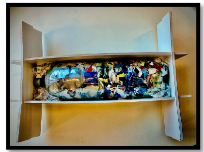
(Author, 2019, 1:1 model demonstrating the eco bricks in the structure)
