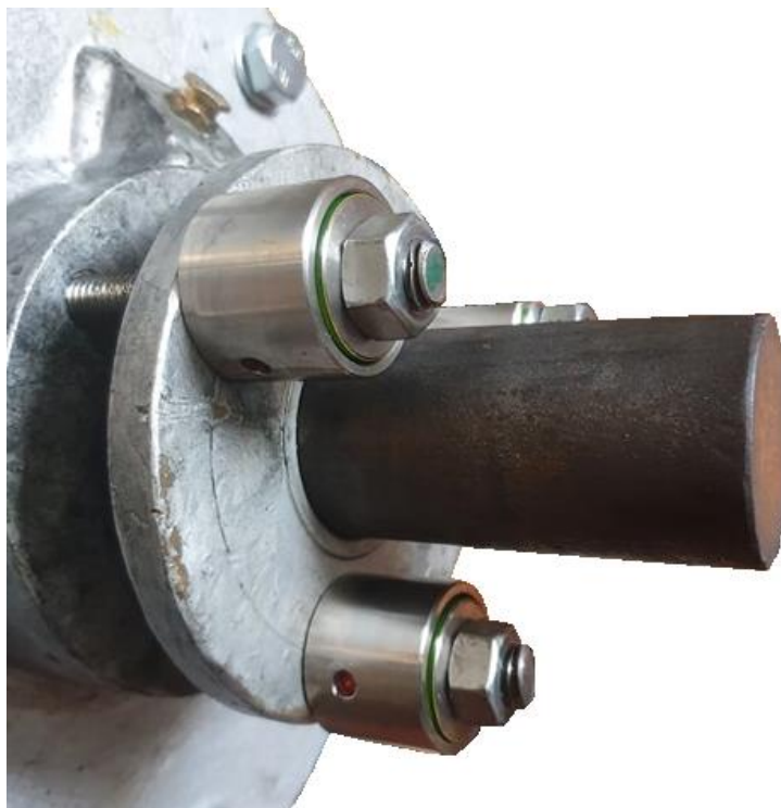
Figure 41 - Removal of M5 Bolts (transferral of load)
