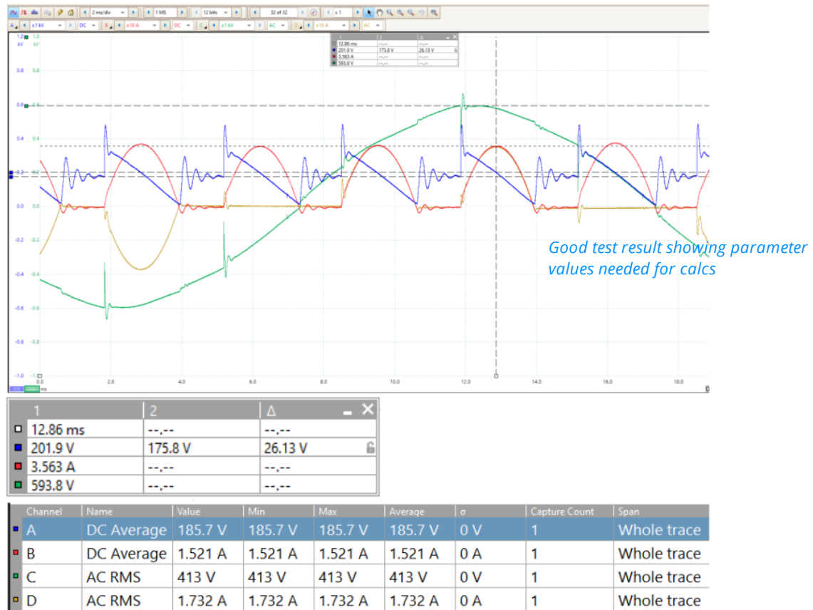
Figure 25 - Motor Constant Pico Scope Waveform and Cursor Tables
