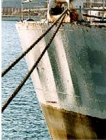
Figure 8. Dishing welding distortion of the steel plate (Universal Technical Institute (UTI), 2019).
