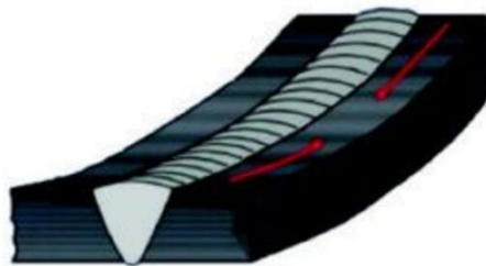
Figure 7. Bowing shrinkage welding distortion (Correia, 2025).
