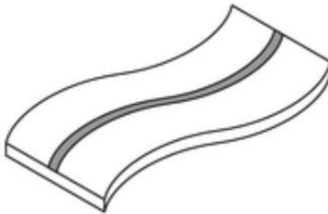
Figure 9. Buckling welding distortion (Barsoum, et al., 2015).
