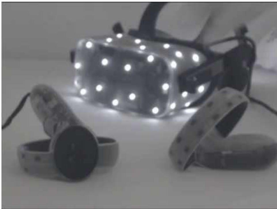
Figure 5: The Oculus Rift headset and controller under infra-red light, showing the infra-red LED's on both [39].
