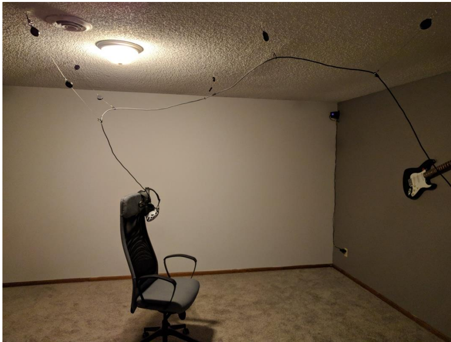
Figure 7: HTC Vive headset using ceiling mounted cables to overcome the majority of the movement and immersion restrictions offered by tethered headsets
