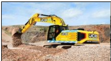
2020 – JCB 220X Hydrogen fuel cell excavator on test.
