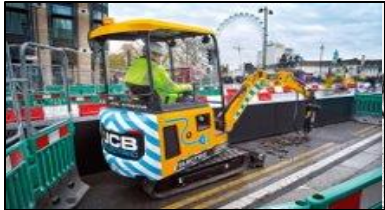
2018 – JCB 19C-IE First electric mini excavator.
