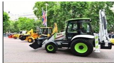
2022 – JCB Backhoe with hydrogen combustion Engine demonstrates at Jubilee Pageant.
