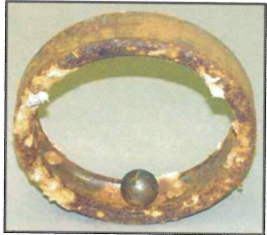
Bearing showing water damage
