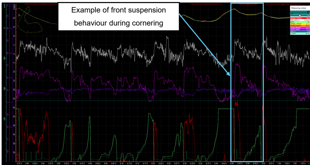
Figure 14: Graph of Brake Pressure, Suspension Travel, Acceleration in x Throttle, Front Brake and Speed of Fastest Lap Session 2 with Example of Front Suspension Behaviour During Cornering Highlighted
