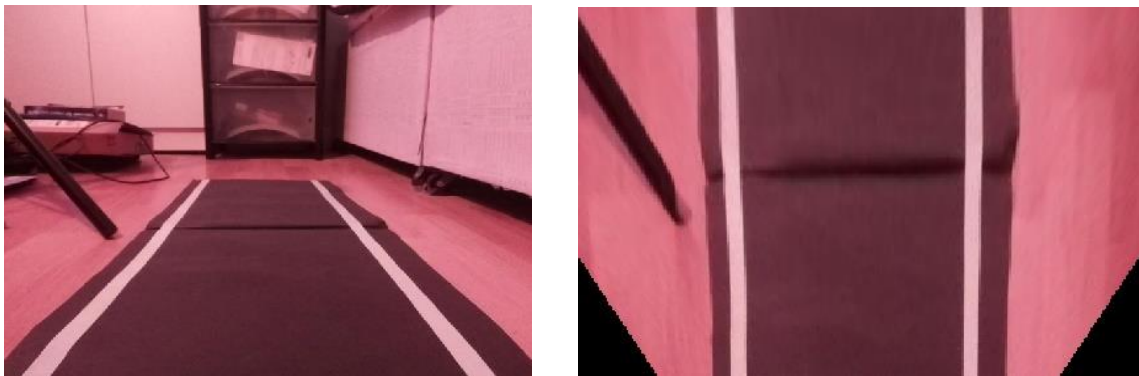
Figure 97 – Original Camera Image (Left) & Transformed Bird's Eye View (Right)
