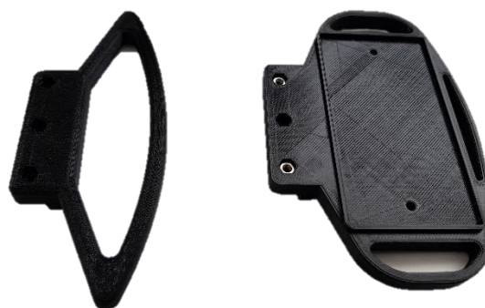
Figure 63 – Different Iterations Of The Rear Bumper; Original (Left) & Modified (Right)
