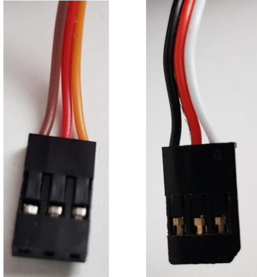
Figure 69 – Connections To Servo Motors; Steering Servo (Left) & Driving Motor (Right)
