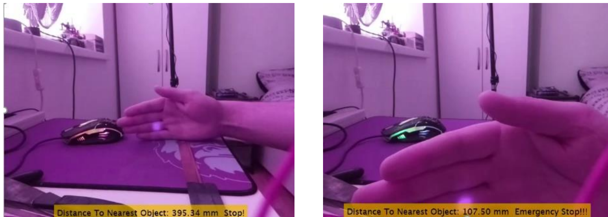
Figure 81 – Testing The Accuracy Of The Infrared Sensor; Object At 400mm Away (Left), Closest Object Could Get To The Sensor (110mm) Before Distance Increased Again (Right)
