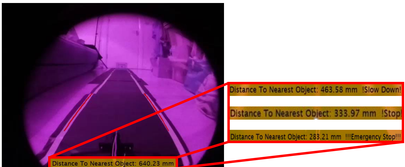
Figure 51 – Distances Annotated Onto The Pi Camera Live Feed Before Setting Specific Values For Each Protocol
