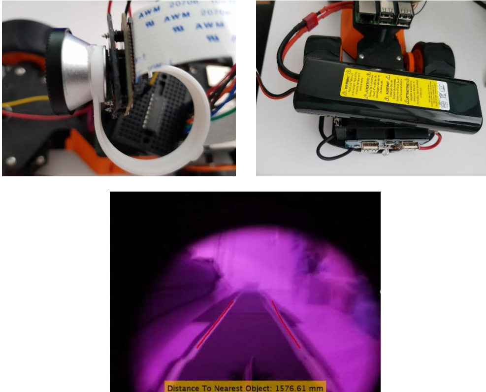
Figure 64 - Fisheye Lens; Attached (Top Left), Motor's R/C Battery Pack (Top Right), Camera Lens Vibration (Bottom)
