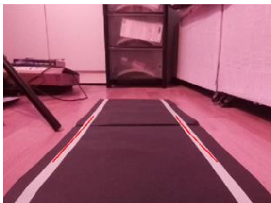
Figure 106 – Parabolic Lanes Annotated Onto The Original Cameras' Image
