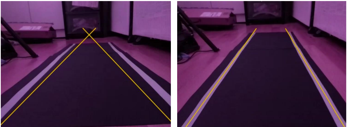
Figure 32 – Physical Testing Using A Camera Mount With 0^\circ To The Vertical; Static Position (Left) & Raised Rear (Right)
