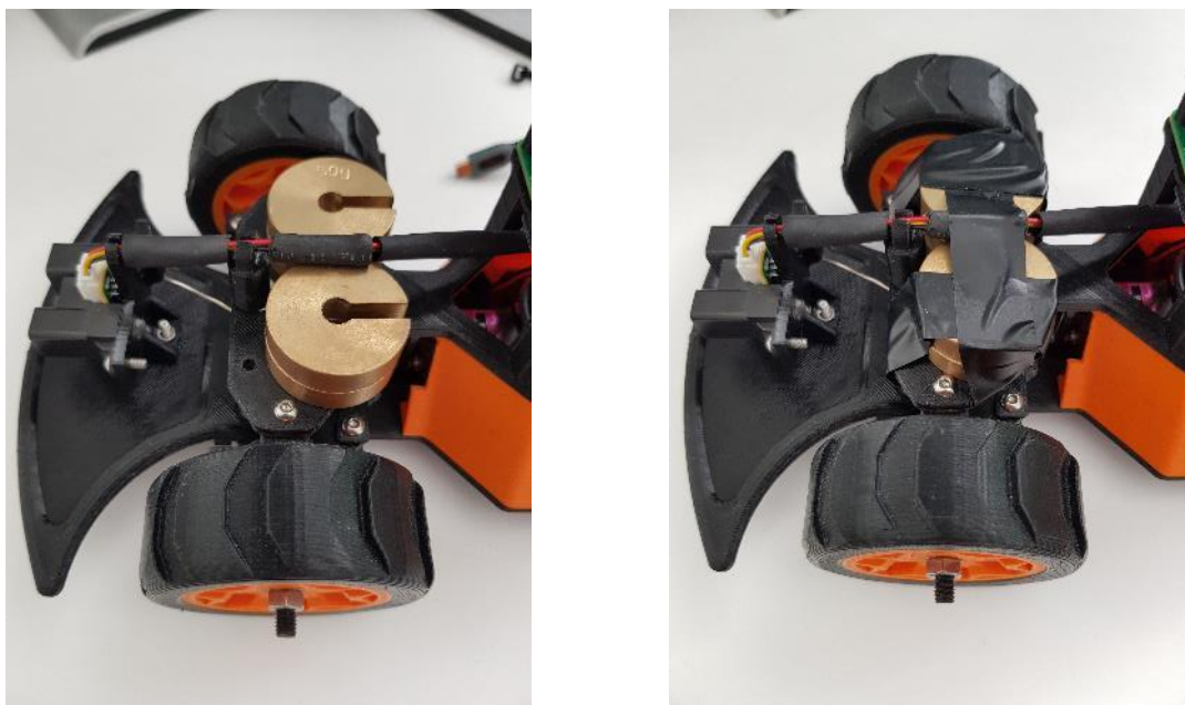
Figure 68 – Weights Used To Apply Downforce To The front Wheels Of The Ego Vehicle, In place (Left), Attached Using Insulation Tape (Right)
