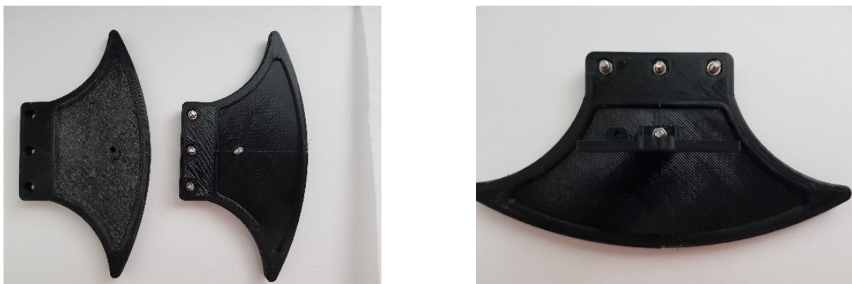
Figure 90 – New Bumper vs. Original (Left), New Bumper Design With Infrared sensor Mount Repositioned
