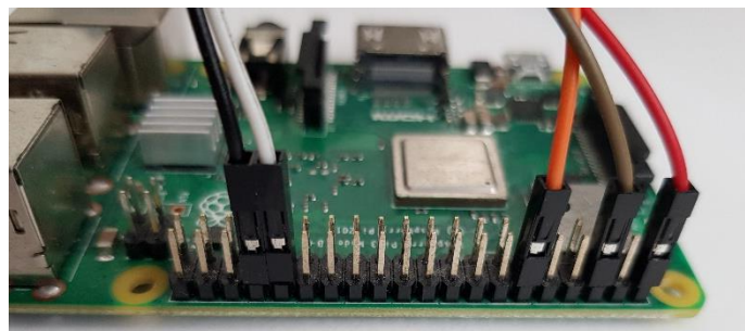
Figure 71 – Both Motors Connected To The Raspberry Pi GPIO Pins
