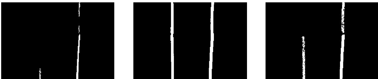
Figure 27 – Effect Of Changing The Lane Marker Size Within The Code, While Keeping The Same Sensitivity Value Of 0.35; 0.01m (Left), 0.013m (Middle) & 0.016m (Right)
