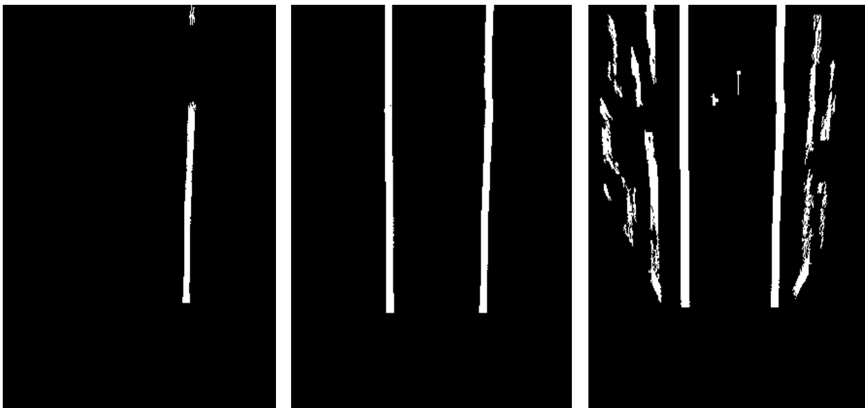
Figure 17 - Changes To The Sensitivity Factor; Too Low (Left), Optimal (Middle) & Too High (Right)
