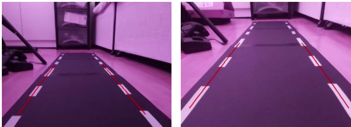
Figure 35 – Effect From Changing The Pitch Of The Camera Mounting; 11.25^\circ (Left) & 22.5^\circ (Right)
