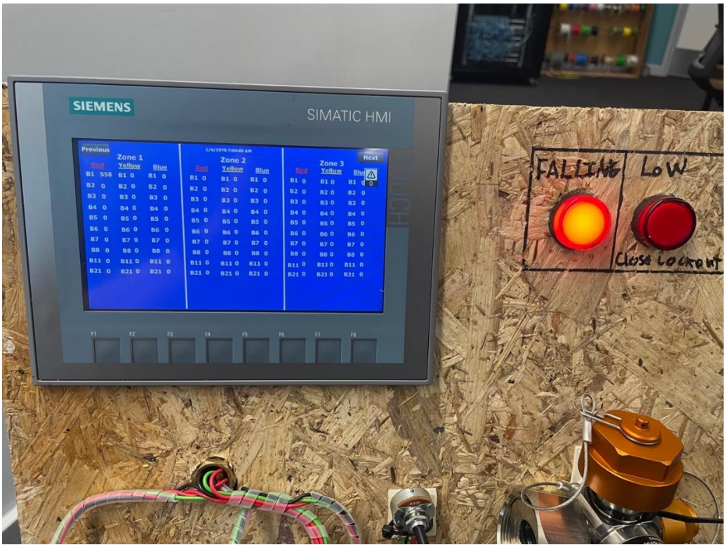
Figure 33: Zone values screen showing the falling SF6 density value
