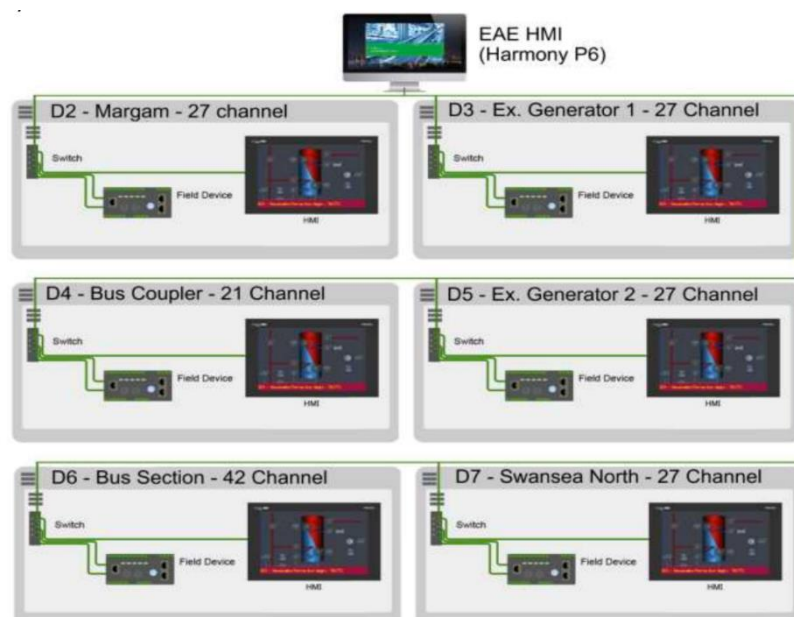
Figure 14: Proposed Schneider Ecostruxure Architecture
