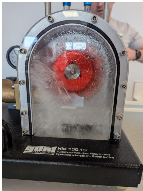
Figure 13 - Pelton Wheel Speed Above Optimal Speed
