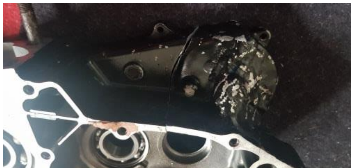
Figure 4 – Crankcase with cracked housing..
