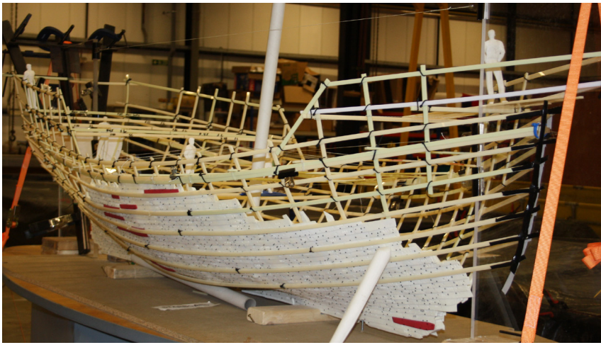
FIGURE 1. THE PHYSICAL SCALE MODEL TWISTED TO MATCH THE FAIRED DIGITAL HULL SHAPE WITH FAIRING RIBBANDS FITTED AT EVERY 4TH STRAKE RUN.
