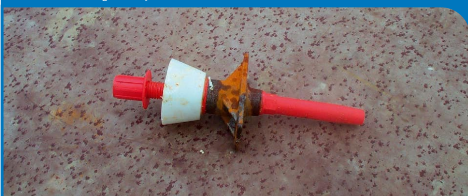
An unbonded anchorage. Courtesy of Balvac.
