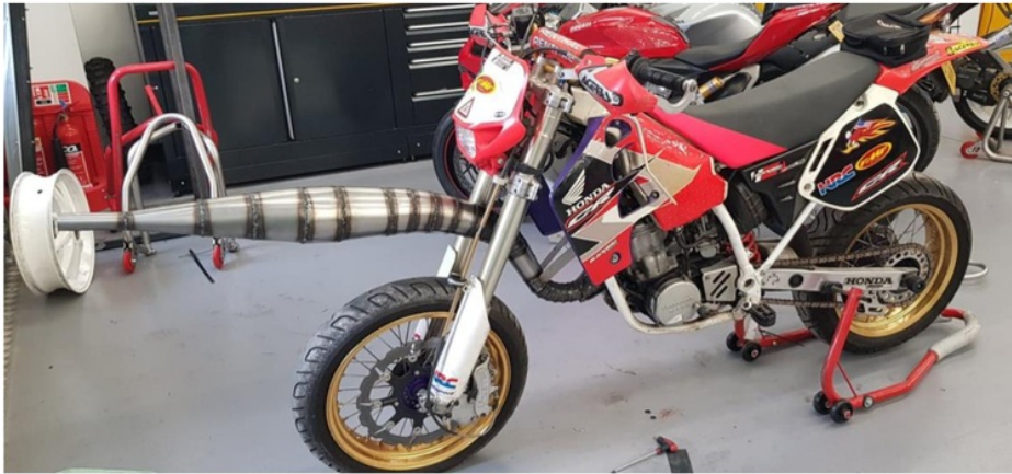
Figure 35 – Manufactured exhaust fitted to CR500R ready for dyno testing. (Parsons, authors own)
