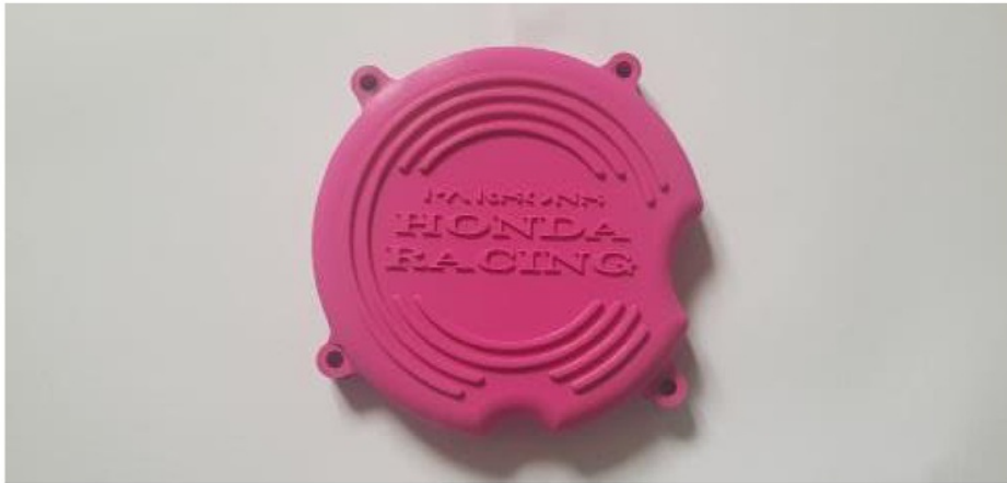
Figure 11 - 3D printed generator cover. (Parsons, authors own)
