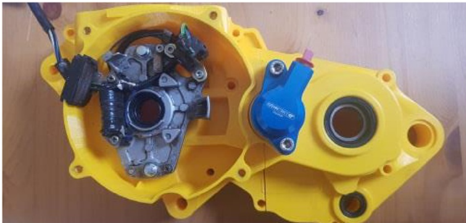
Figure 11 - 3D printed generator cover. (Parsons, authors own)
