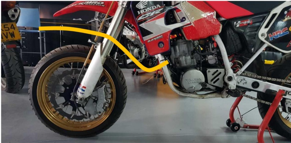
Figure 26 – Side on photograph of the CR500R with suggested exhaust routing shown in yellow.
