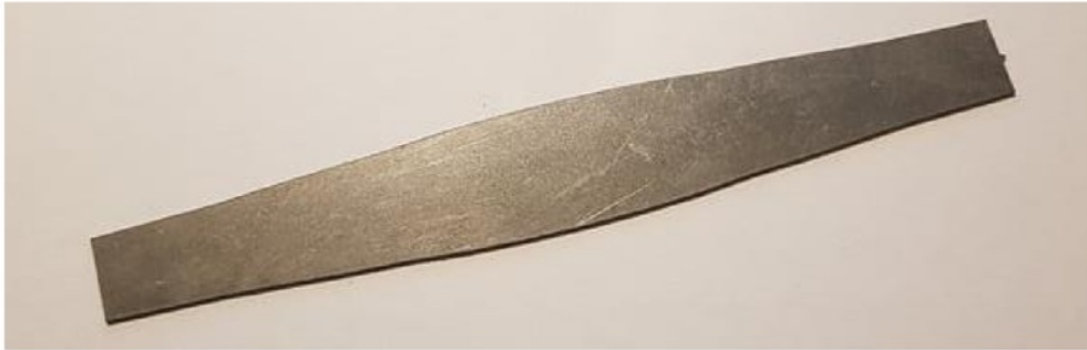
Figure 31 – Photograph of a Lead-In pipe segment. (Parsons, authors own)
