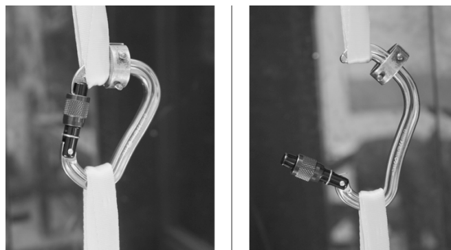
Figure 4.0.3 - test two, loading the carabiner at an offset from its major axis at points B and C. This configuration deformed at 10.63KN (Black Diamond, 2016)
