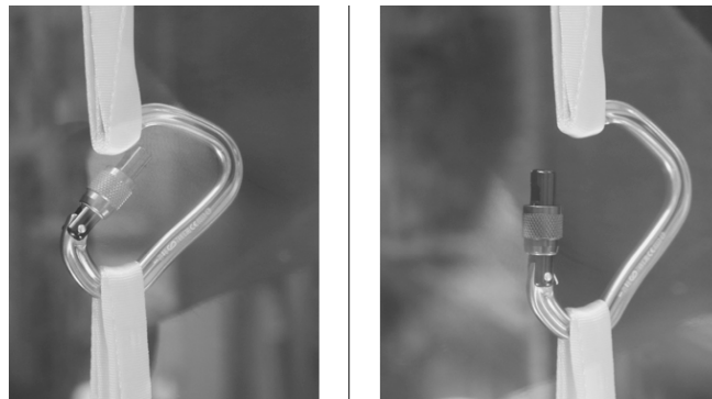
Figure 4.4 – test 3, loading the crab from the nose of the locking gate, the furthest point from the major axis. Deformation was seen after just 5.21KN (Black Diamond, 2016)
