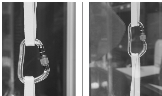
Figure 4.0.2 - Test one, loading the carabiner through its major axis. The crab took a load of 21.8KN before deformation was seen (Black Diamond, 2016)
