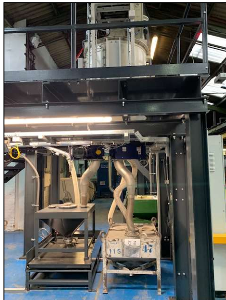
Figure 61 - Air Classifier Hopper Collection
