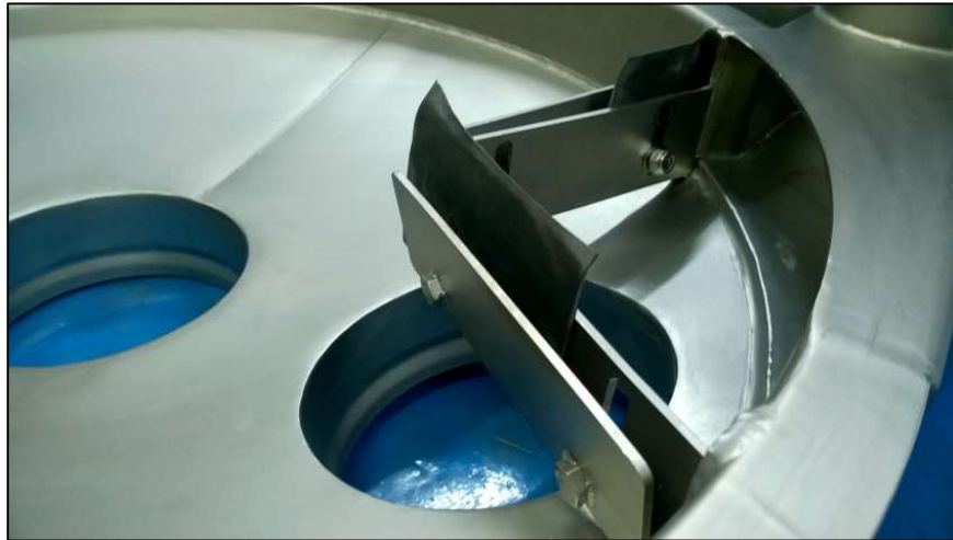
Figure 31 - Powder Scraper on the Virto Screener
