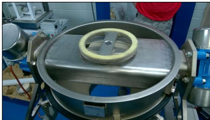
Figure 30 - Beater Ring of the Virto Screener
