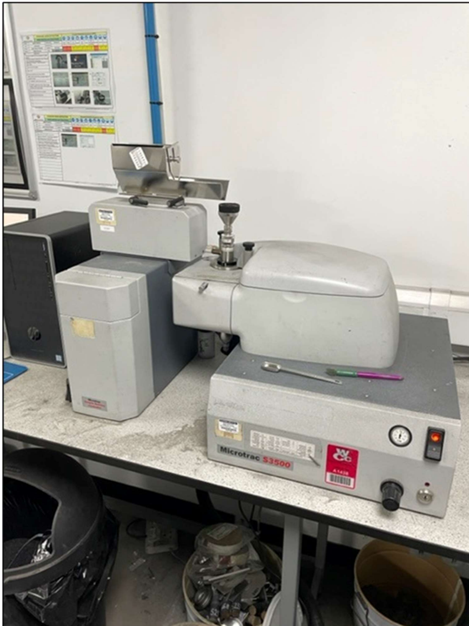
Figure 16 – Laser Diffraction Analyser at Wall Colmonoy
