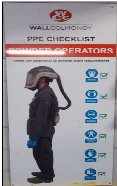
Figure 36 - PPE Requirement For Screening Powder
