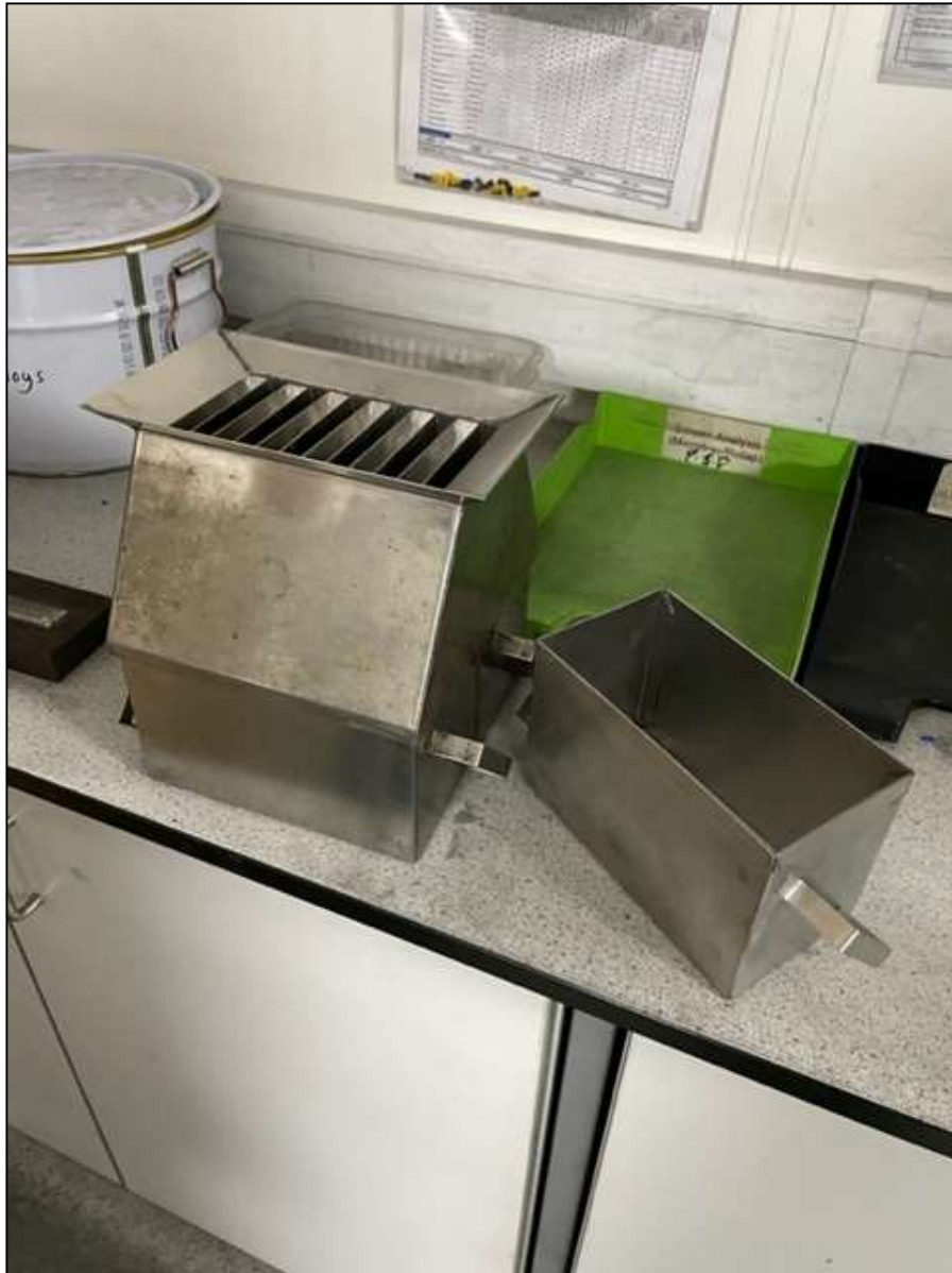
Figure 21- Riffler Used at WCL
