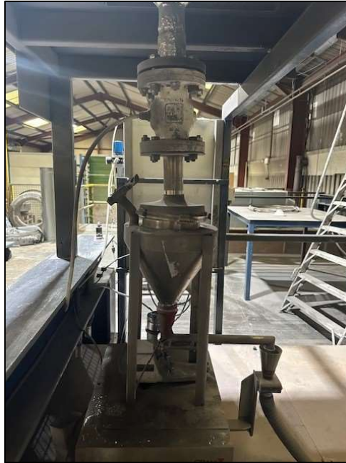
Figure 26 - Pinch Valve LIW Feeder at WCL
