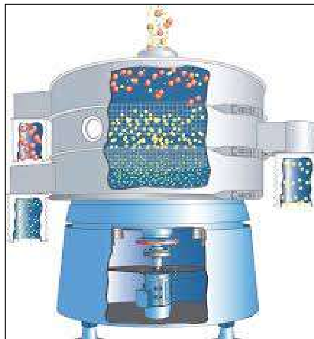
Figure 9 - Vibratory Screening Schematic, Courtesy of, (Kay, 2010)
