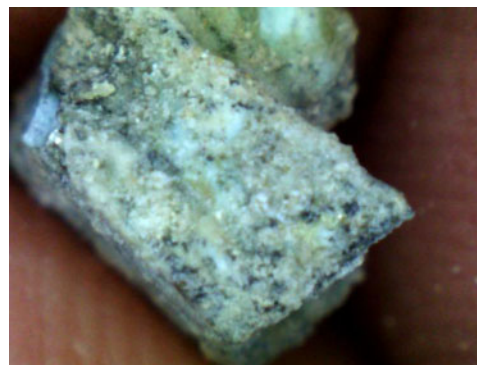
6 The internal material of the faience beads consists almost completely of interstitial glass. No clay core is visible. This is typical for the efflorescence method, used in Egypt (photograph A. Giumlia-Mair)
