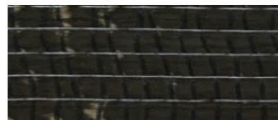
Figure 1 - unidirectional weave example (Boeriu, 2014)
