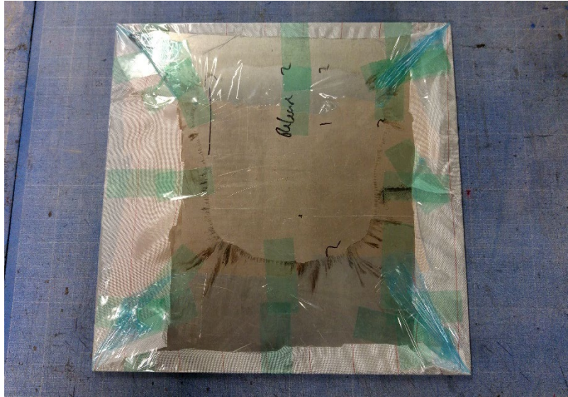
Figure 16 - underside of the autoclave tool, showing peel ply and release film secured
