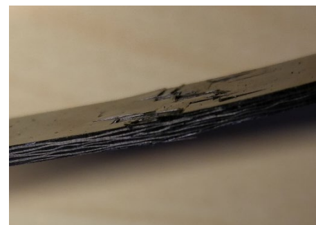
Figure 43 - evidence of compression fracture of the outer surface is visible, along with possible interlaminar shear
