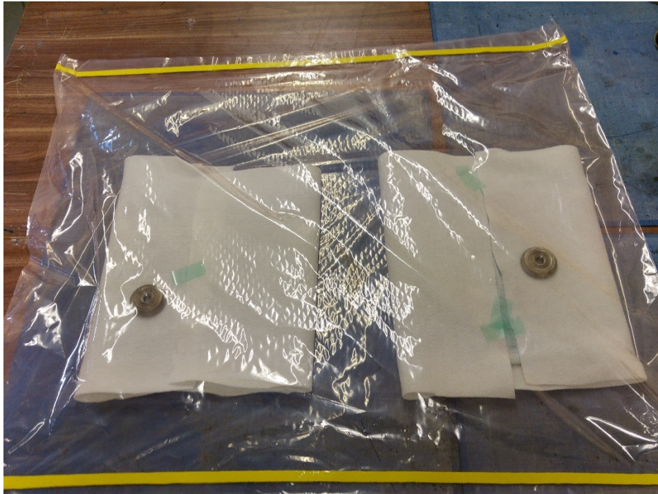
Figure 18 - shows both sides of the vacuum bag sealed, and the vacuum valves in position on the breather cloth
