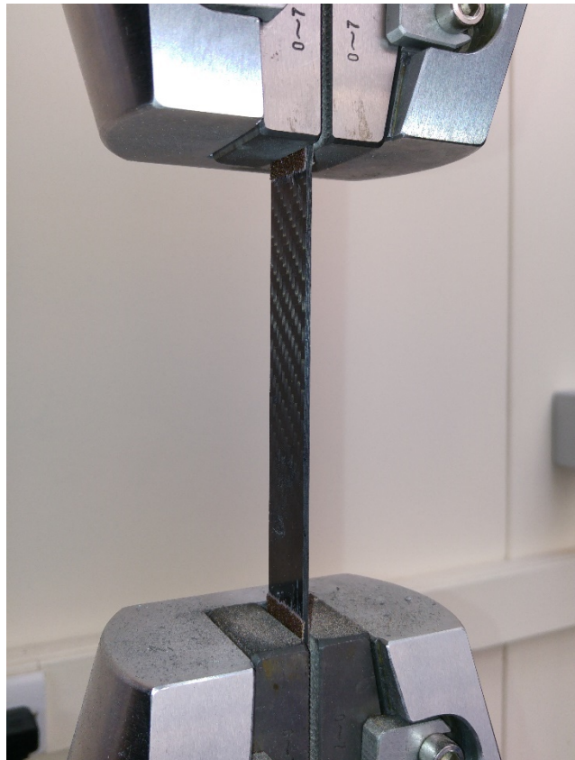
Figure 26 - one of the tensile specimens during testing, note the emery cloth tabs between the self-tightening grips and the specimen
