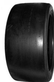
Figure 13 – Avon A53 (11851) slick racing tyre [33]
