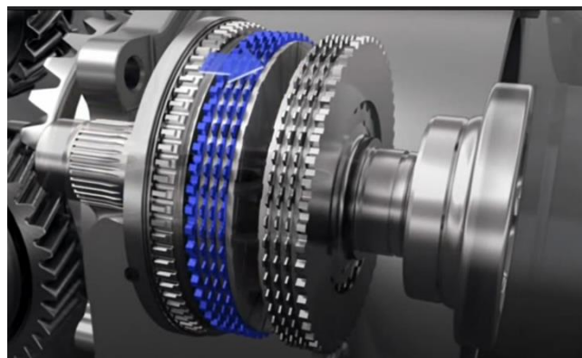
Figure 6- Torque vectoring clutch packs (Ferrari, 2011)
