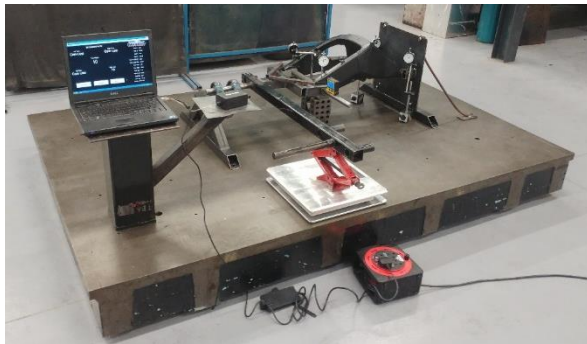
Figure 10. Stiffness experiment to the original swingarm
