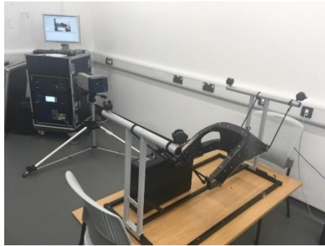
Figure 12. LDV experiment to the original swingarm
