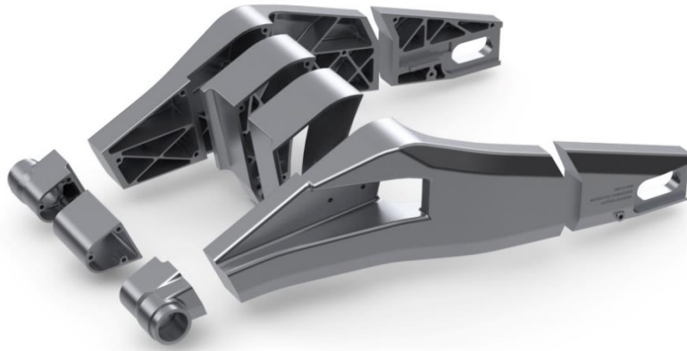
Figure 75. Final design proposal of the swingarm - exploded view
