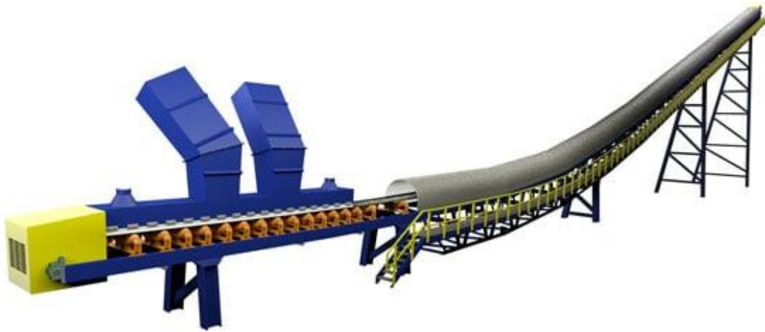
Figure 1.2: Coke Belt Conveyor with Weather Covers (Feeco, 2023)
