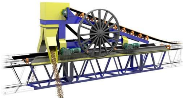
Figure 1.4 Belt Tripper with Diverter Chutes (Feeco, 2023)
