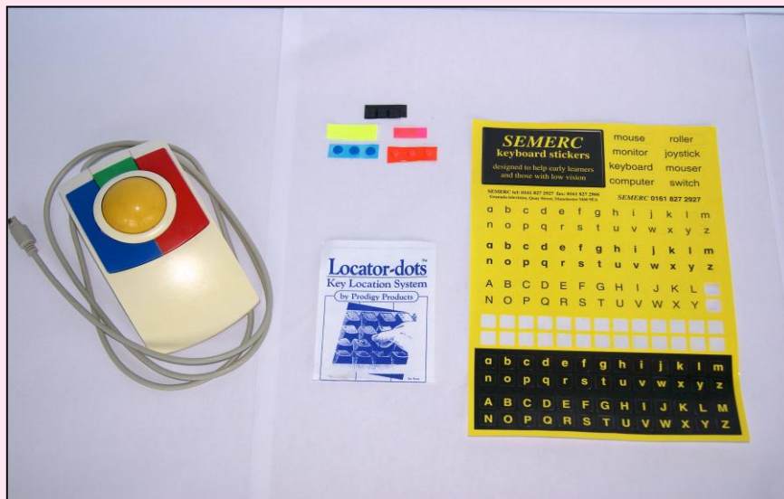
Fig 7 An adapted mouse for the computer which has been enlarged and coloured. Coloured 'Bumpy Lumps' and locator-dots to stick on to key boards. Coloured and enlarged letter labels for computer keys.
