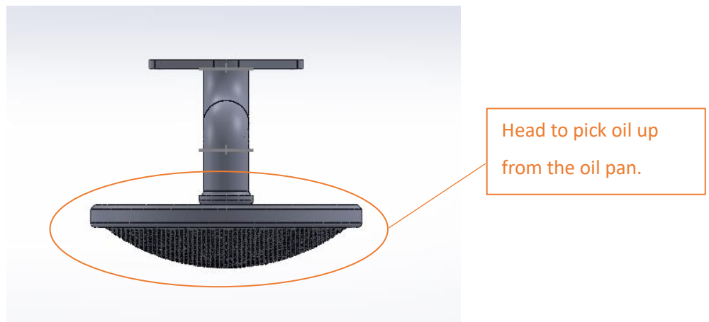
Figure 19: Front view of oil pick-up pipe.
