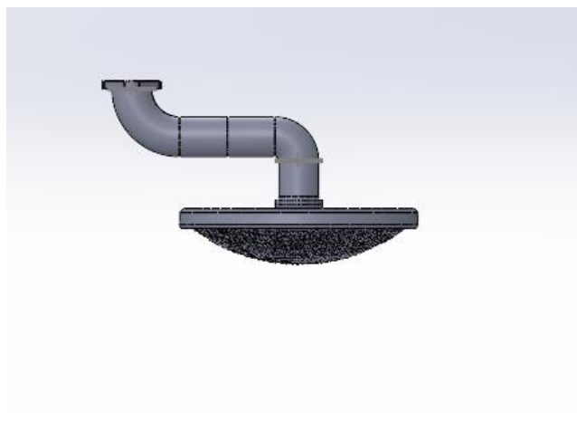
Figure 20: Right view of oil pick-up pipe.
