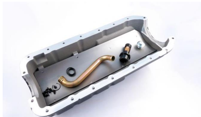
Figure 7: Existing dry sump pan 3.
