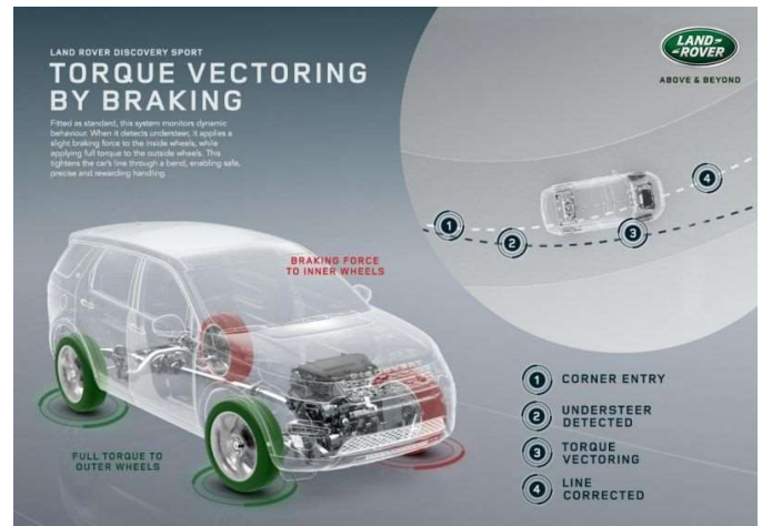
Figure 4: Land Rover Discovery Sport Torque Vectoring (Shah, 2021)
