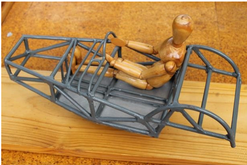
Figure 1 - a model of the chassis using a mannequin illustrating the form and function of the tub.
