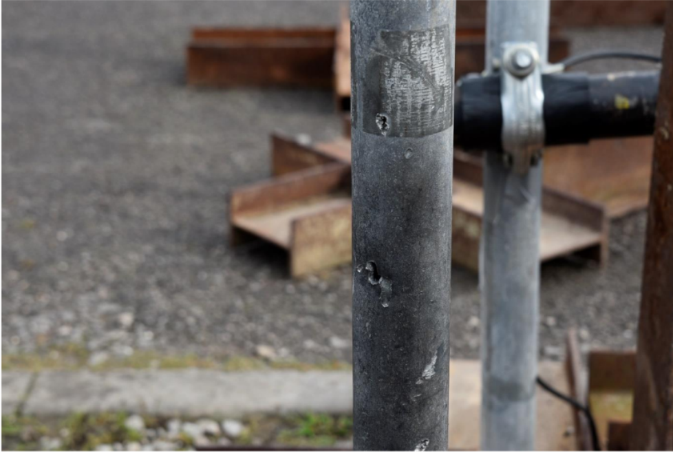
Figure 12 - post-firing pressure gauge stand (1m) carbon deposit.
