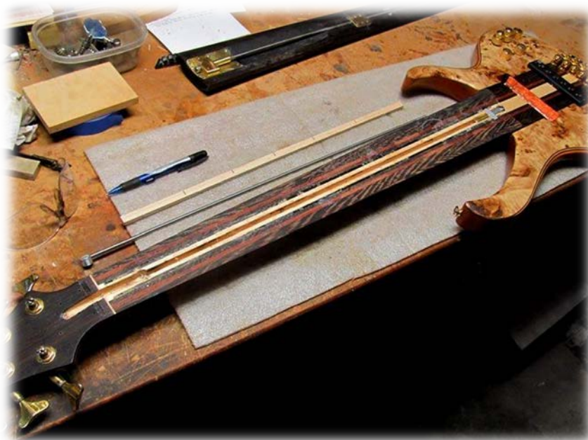
Fig. 4 guitar with the fretboard removed, showing the cut for thruss rods. Here: truss rods replacement.
