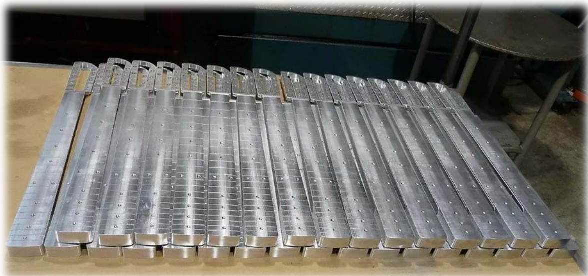
Fig. 7 Guitar necks machined from aluminium billets.
