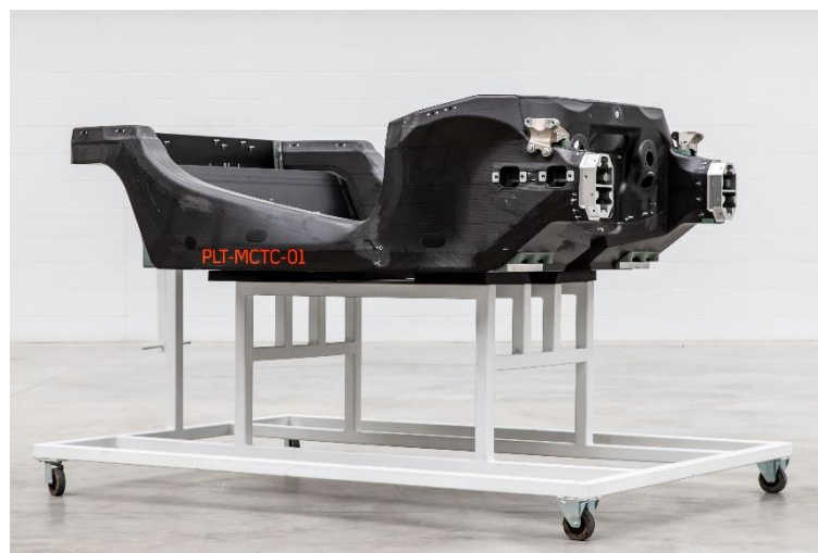
Figure 10 - Carbon Fibre Monocoque (McLaren Automotive, 2019)
