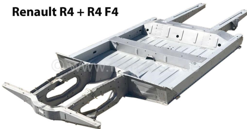
Figure 4 - Renault 4 Platform Chassis (der Franzose Automobiltechnik GmbH, n.d.)
