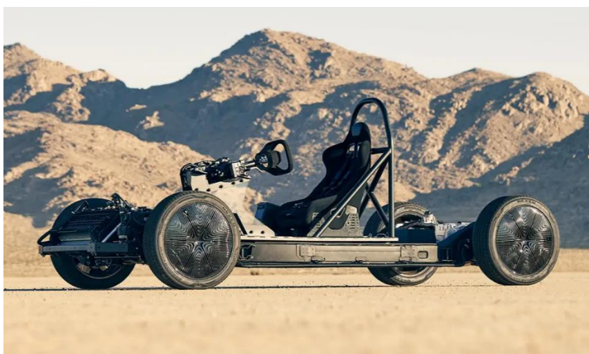
Figure 14 - Canoo Electric Skateboard Platform (Canoo, n.d.)
