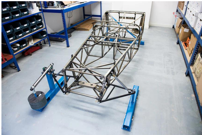
Figure 6 - Caterham 7 Triangulated Frame (Motortrend, 2016)
