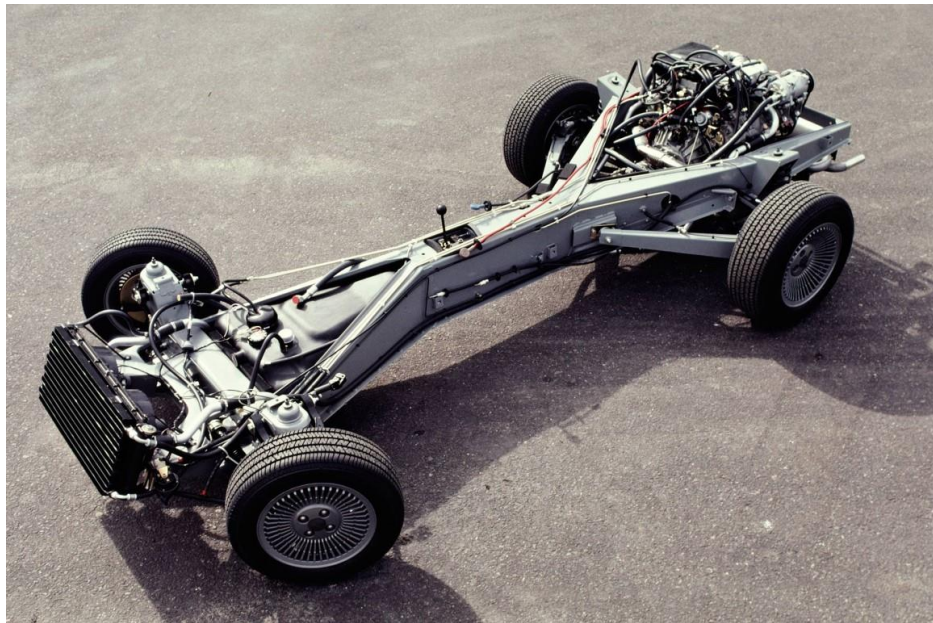
Figure 5 - DeLorean DMC-12 Chassis (DeLorean Directory, n.d.)
