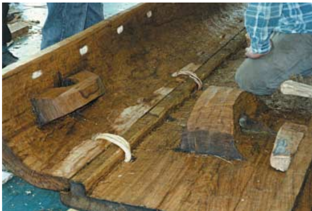
Figure 8. A full-size cross-section of the strange construction was replicated from green oak using copies of Middle-Bronze-Age-tools. The ile , or curving plank between the bottom and (missing) side, can be seen together with two chunky cleats carved out of the solid. (V. Fenwick)
