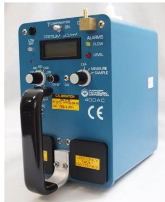
Figure 5.4 - Overhoff 400 tritium in air monitor
