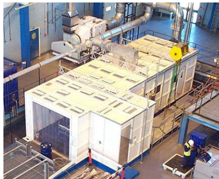
(b) Modular containment structure
