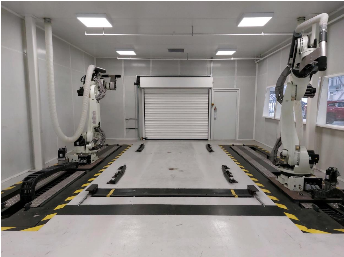
Figure 2 - Internal view of the wind-noise rig showing dual robot arrangement
