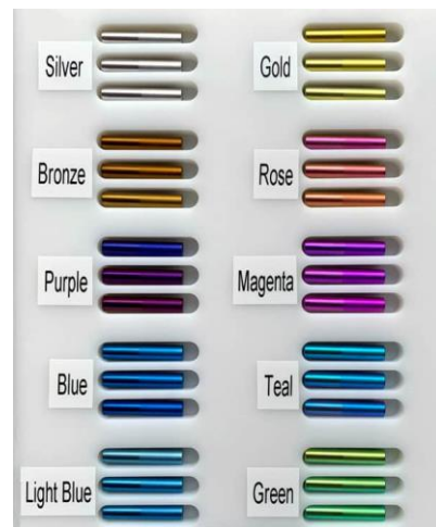
Figure 6 – Titanium anodizing colour chart [10]
