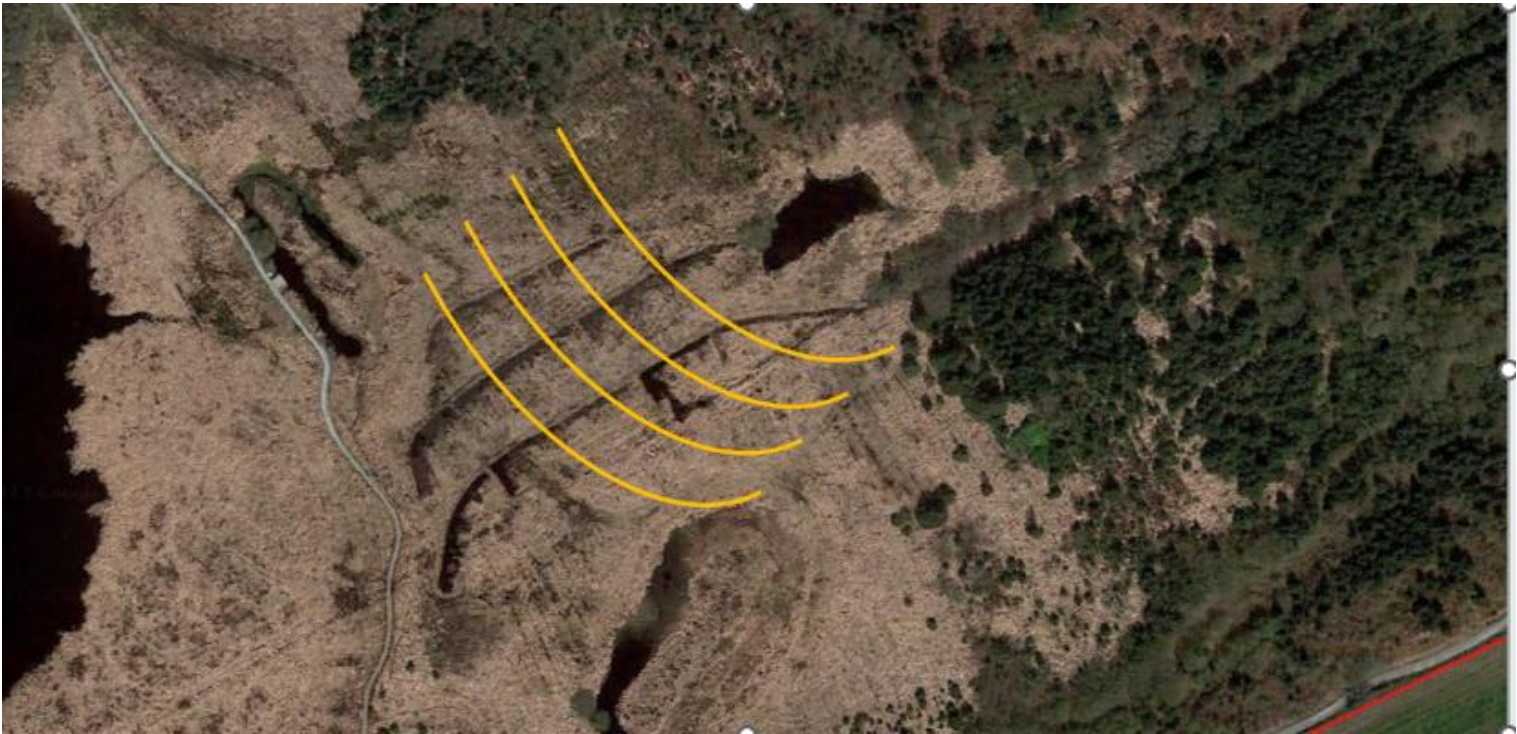
Figure 14 Example of correct bund positioning Image Source: Google Satellite. Annotations Egan, (2023)
