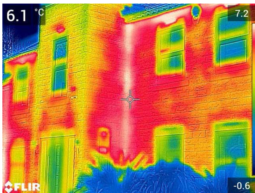
Figure 3.1 Infrared image capturing radiation emissions and transposing the data to visible light, referencing to the colour scale on the right
