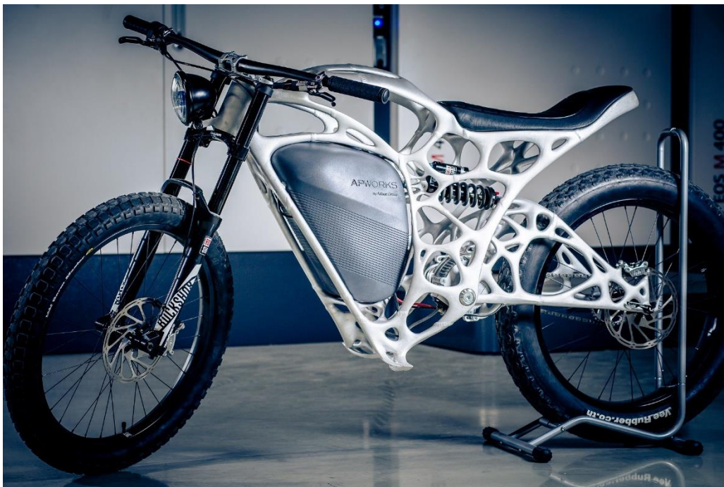
Figure 4 - shows a motorbike that as been topology optimised to have as little material as needed. (motorbikeIMG, 2024)
