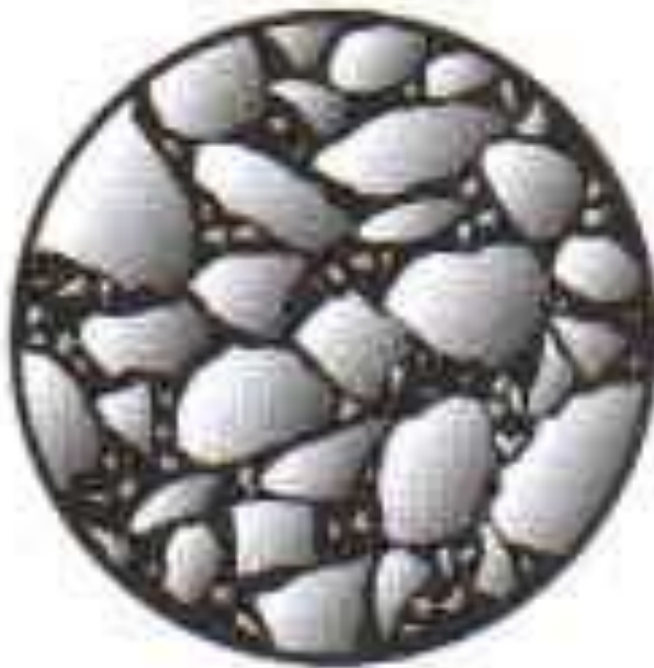
Stone Matrix Asphalt SMA
