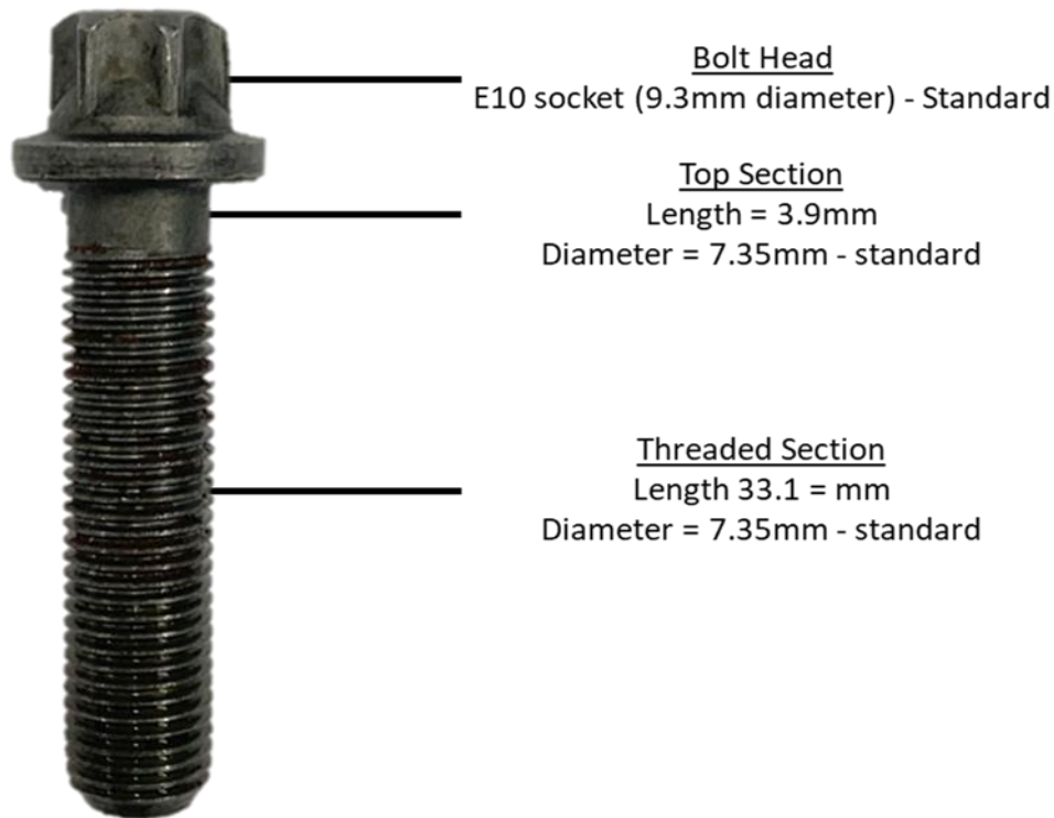
Figure 18 - Standard Con-rod Bolt Design (Hart, 2020)
