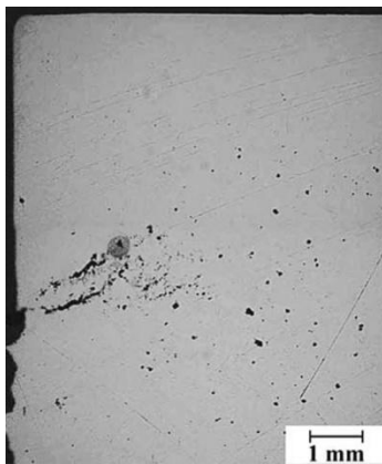
Figure 2 Voids in a cast Metal due to Cooling (Otarawanna, et al., 2009)
