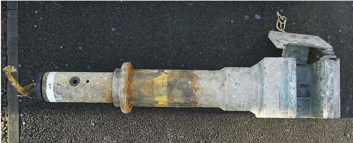
Figure 15-12 Pyromechanical cable cutter designed for a deep sea environment (Courtesy of Chemring Energetics Ltd)
