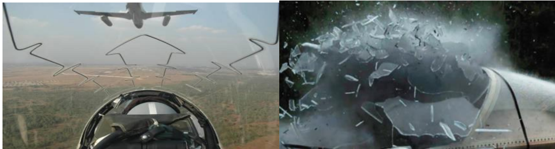
Figure 15-6 Miniature detonating cord (MDC) can be seen attached to the aircraft canopy (left) and completely fragments the canopy as part of the ejection sequence (right) (Courtesy of Chemring Energetics Ltd)
