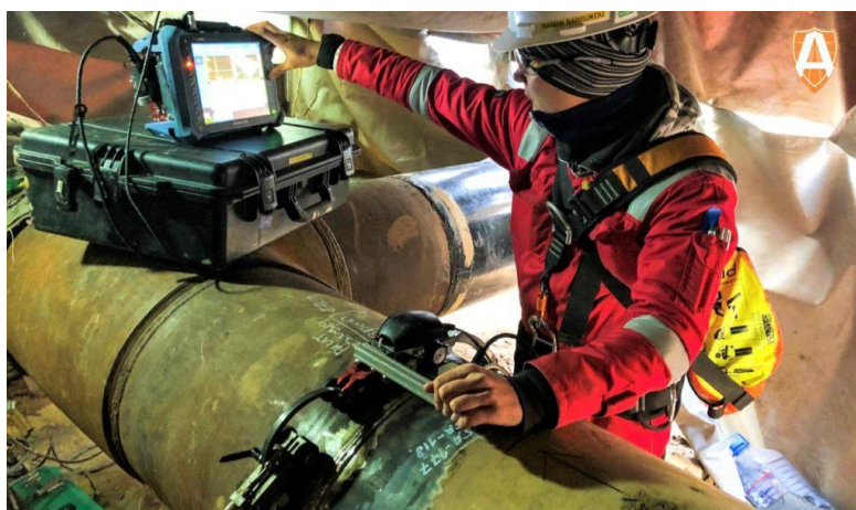
Figure 1: Phased Array Ultrasonic Testing (PAUT) ( (arisegobal.com, n.d.)
