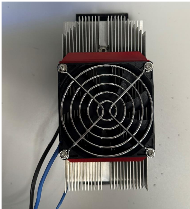
Figure 15 - Rear Side of Thermoelectric Device
