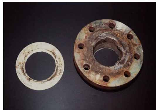
Figure 9: The mechanism of crevice corrosion in metals.
