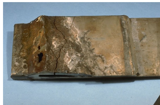
Figure 7: The phenomenon of stress corrosion cracking.
