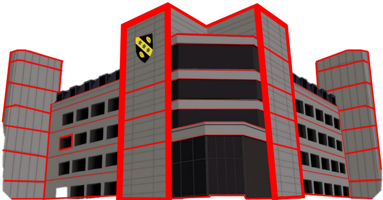
Figure 2.1: RED indicates areas susceptible to cold bridging at the UWTSO Business Campus (Meyrick, 2019)
