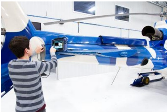
Figure 3: Image of test technician performing ultrasonic NDT test on a helicopter tail (Olympus, 2019)
