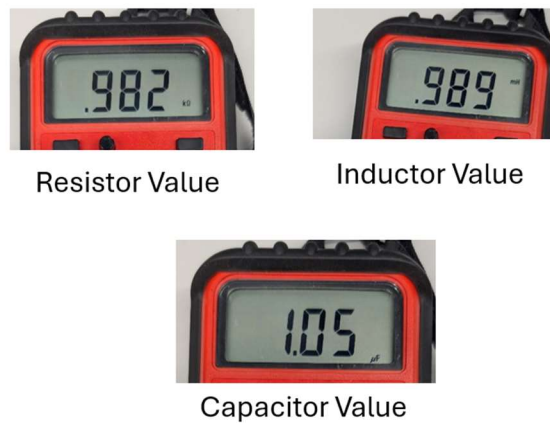
Figure 6: The values of the resistor, inductor and capacitor shown at 982 Ohms, .989 mH and 1.05uF respectively.
