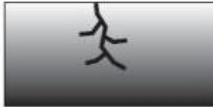
Stress Corrosion Cracking
