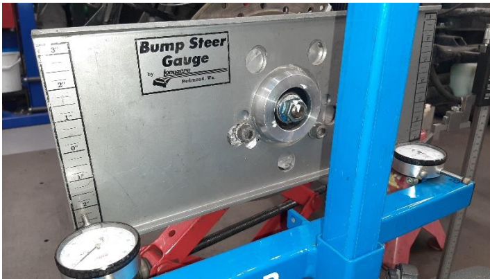
Figure 9 - Bump Steer Gauge
