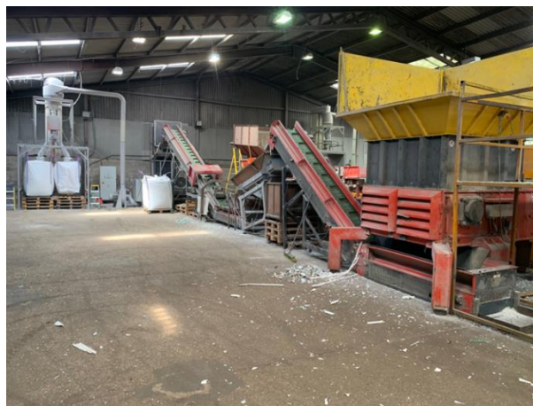
Fig 1. photo take on site visit - Shredding and granulating line at RPCS
